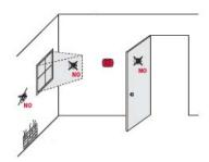
Do not install in locations where the thermostat can be affected by:
