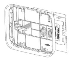
Step 4 Insert the cable into connector on circuit board of thermostat.
